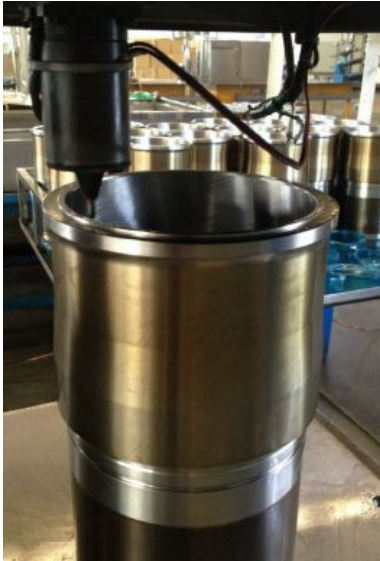
CTP liners are marked on the liner flange spigot top face using the dot peen technology.
